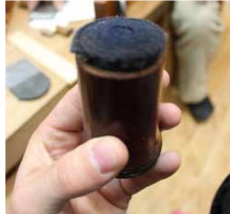
Above: Oil-soaked leather wad used to prevent freshly sharpened irons from rusting Opposite top: experiments and trials in Nakagawa Shuji's studio near Lake Biwa, Kyoto Opposite bottom: the assembly process of Nakagawa's ki-oke bucket base.
